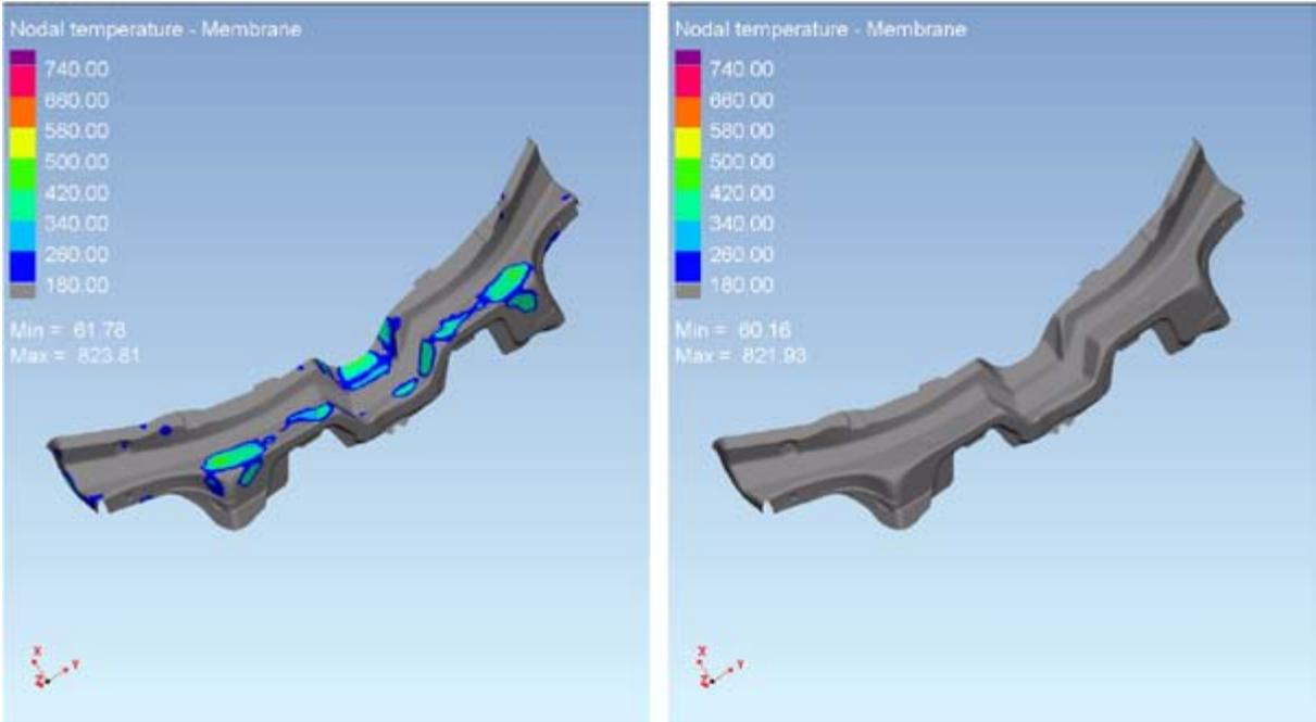
Fig. 9: Temperature at the end of quenching – Spotted (right) and not spotted die face
