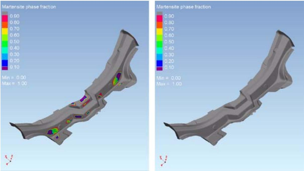
Fig. 10: Martensite formation at the end of quenching – Spotted (right) and not spotted die face
