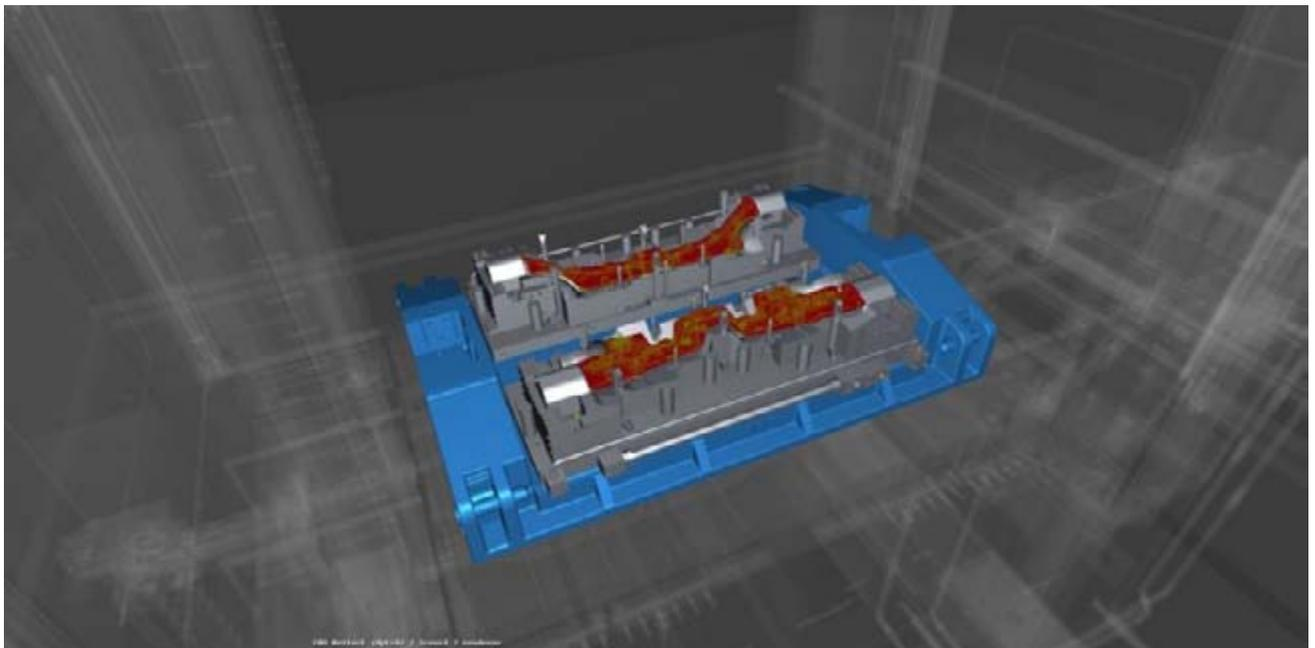
Fig. 13: Blank temperature displayed in the production line in the virtual reality system IC.IDO
