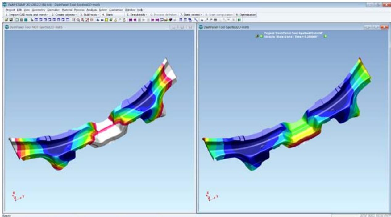
Fig. 11: Distortion after cooling on air – Spotted (right) and not spotted die face
