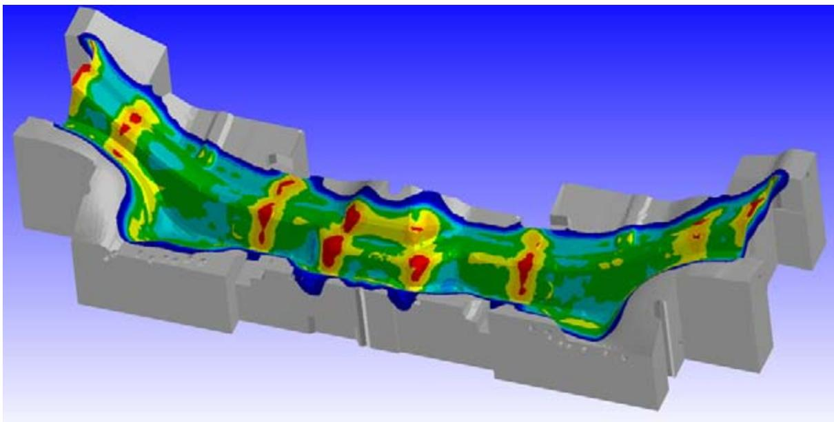
Fig. 12: Die face temperature after a few cycles – initial design with temperature peaks. The final design does not show those peaks any more.
