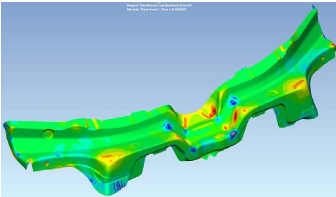
Fig. 6: Percent thinning versus nominal blank thickness
