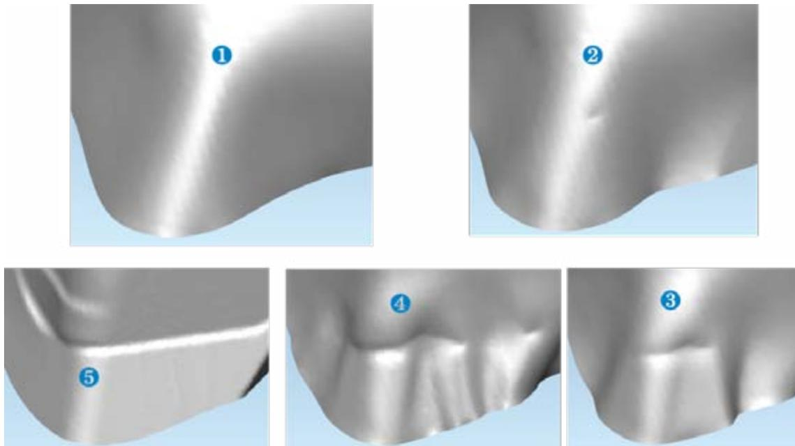
Fig. 7: Evolution of wrinkles during forming
