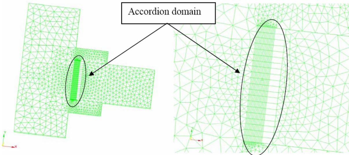
**Figure 5:** Automatic generation of the accordion domain. The thickness of the elements is set here to a small value to make the elements visible. One layer of elements of the accordion domain is already stretched (POST project, [18]).
