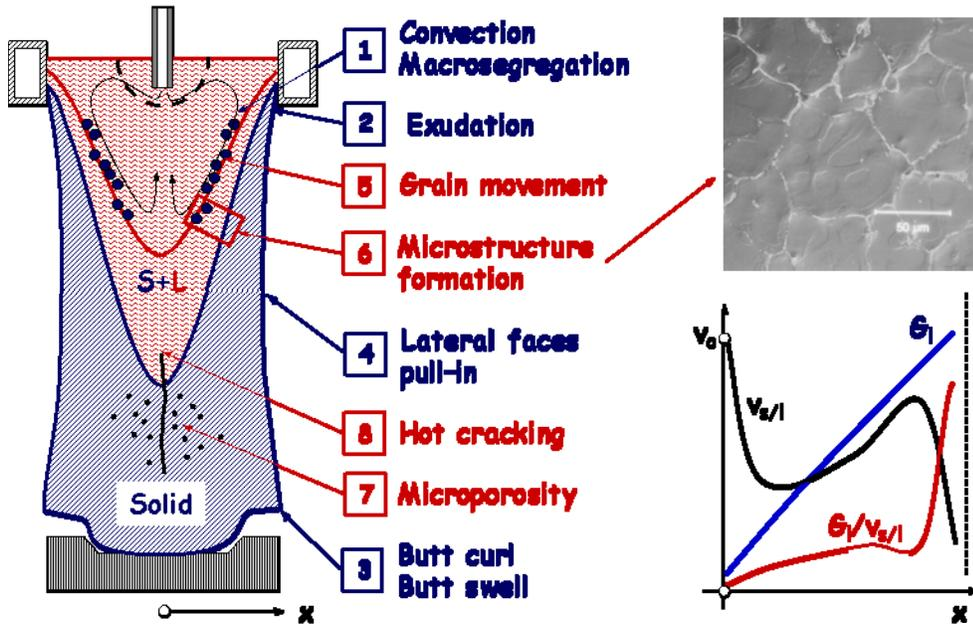
**Figure 1:** Schematics of the VDC casting process. Topics 1-4 correspond typically to a macroscopic approach, whereas topics 5-8 correspond to a microscopic one. Typical variations of the thermal gradient,  $G$ , of the solidification rate,  $v$ , and of  $G/v$  are shown as a function of  $x$  [1].
