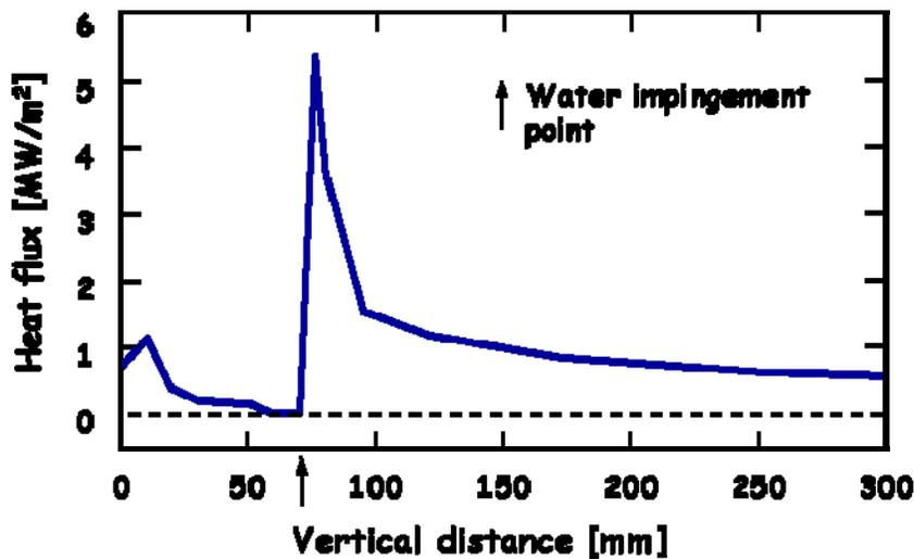
Figure 2: Computed heat flux as a function of the distance to the top liquid level for an AA5182 alloy [4].
