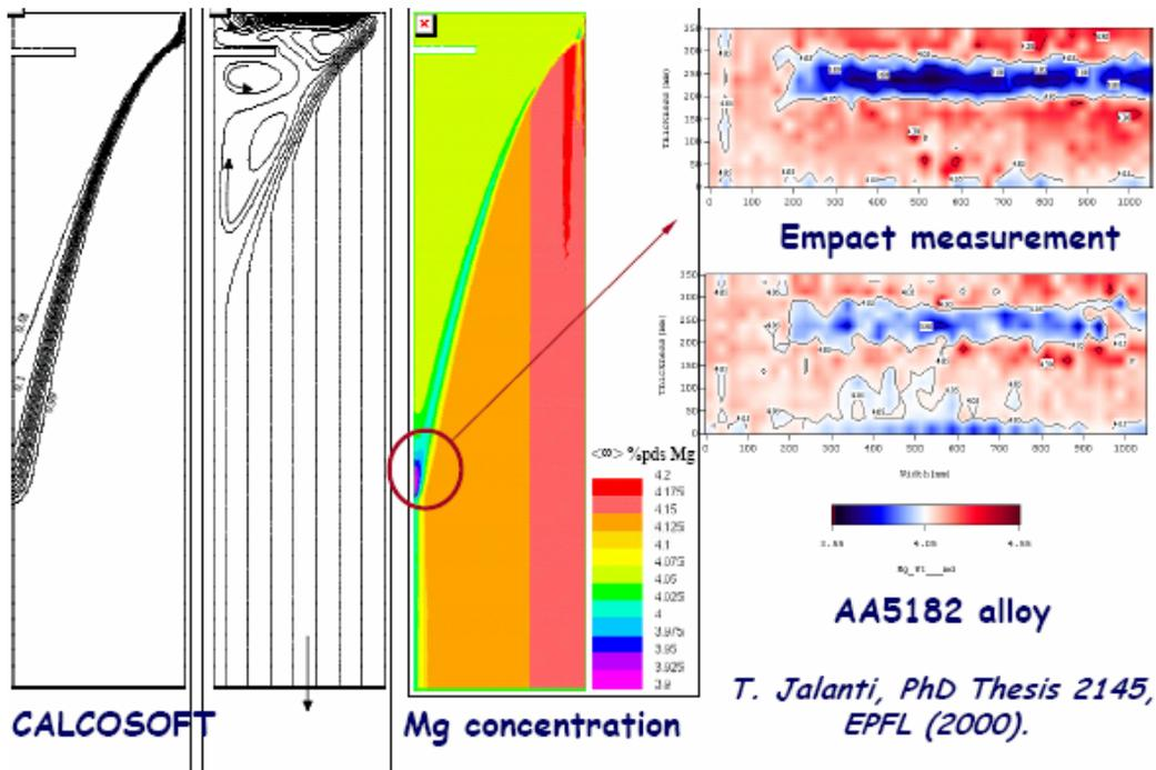
**Figure 4:** Macrosegregation results for a 2D section of an AA5182 DC cast slab, as calculated with the CalcoSOFT software. The various pictures represent, from left to right: the steady state temperature profile, the iso-fractions of solid showing clearly the mushy zone position, the velocity field, the streamlines and the average Mg concentration [16].
