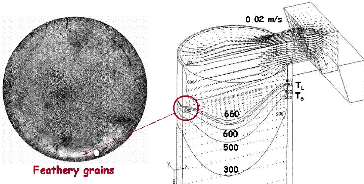
**Figure 3:** Velocities and temperatures at the surface and in the vertical symmetry-plane for an AA1050 DC cast billet, injected from the lateral side, as calculated with the Fidap software. Temperatures are in °C, ( $T_{liq} = 657$  °C,  $T_{sol} = 645$  °C). In-flow velocity is 0.02 m/s, from [10].
