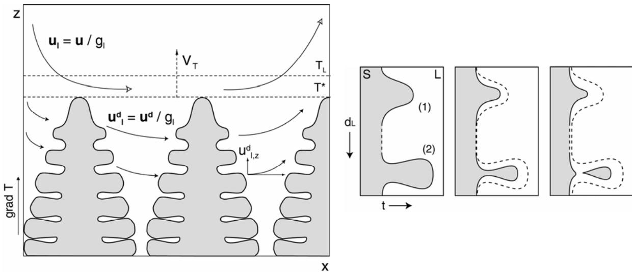
**Figure 6:** Schematic representation (left) of local fluid flow in the liquid,  $u_l$ , and in between the dendrites,  $u_l^d$ . The projection of  $u_l^d$  on the thermal gradient (parallel to the  $z$ -axis),  $u_{l,z}^d$ , has to be compared with the velocity of the isotherms  $V_T$ . On the right, schematics of remelting (1) and fragmentation (2) of secondary dendrite arms [21].
