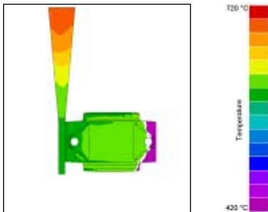
Figure 7: Temperature contours showing the position of the pyrolytic zone after 12.8 seconds (Procast™).
