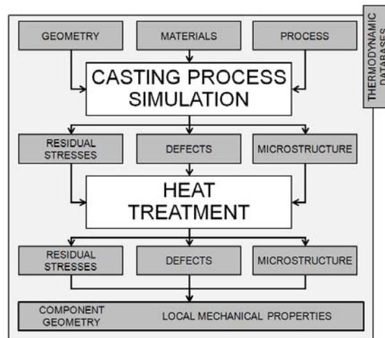
Fig. 8: Casting and heat treatment modelling scheme.
