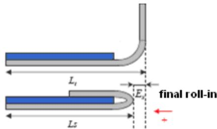
Fig. 4. Final roll-in after the hemming process
