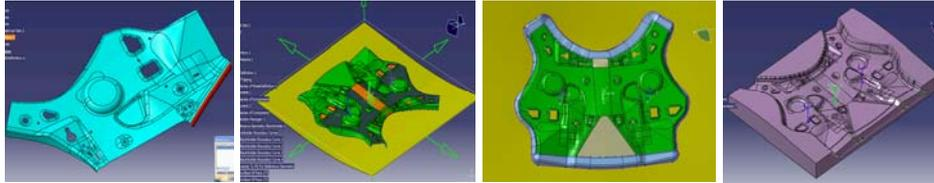
Fig 2. A sample for an integrated die design system; DIEMAKER for CATIA V5; Typical workflow from part over blankholder design to addendum surfaces and finally solid model export.
