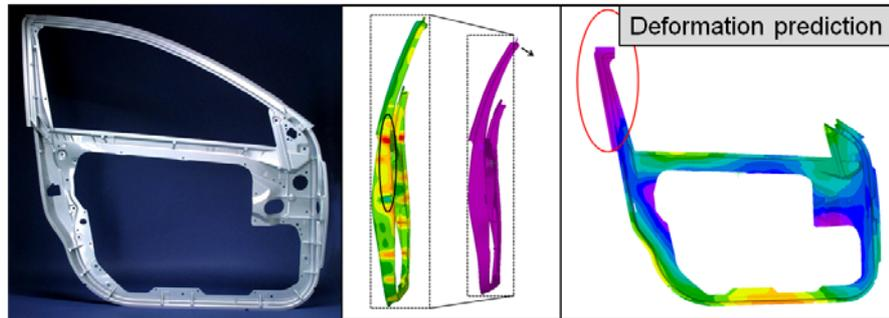
Fig 9: Deformation prediction of a door from Mercedes Benz (Courtesy of +GF+)
