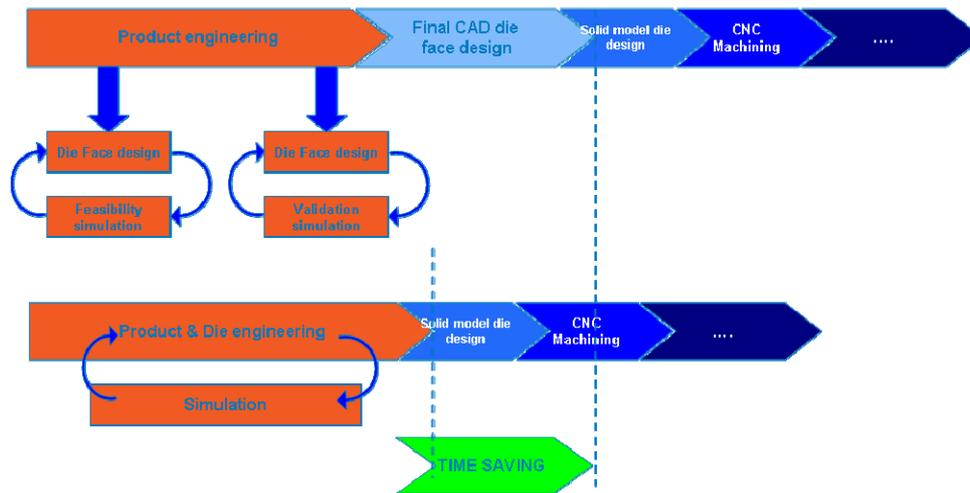
Fig 1. Conventional workflow on top, new proposed workflow based on DIEMAKER for CATIA V5 below – showing clearly the potential time saving.
