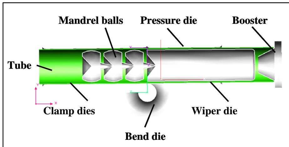
Picture 5: Simulation model mandrel bending
