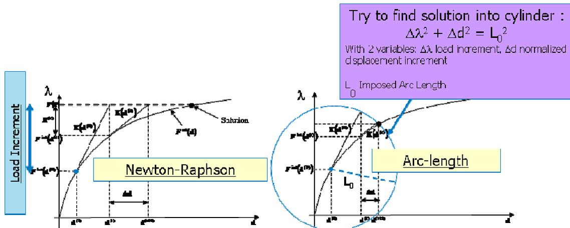
Figure 4: Comparison of the Newton-Raphson method with the Arc-length method.
