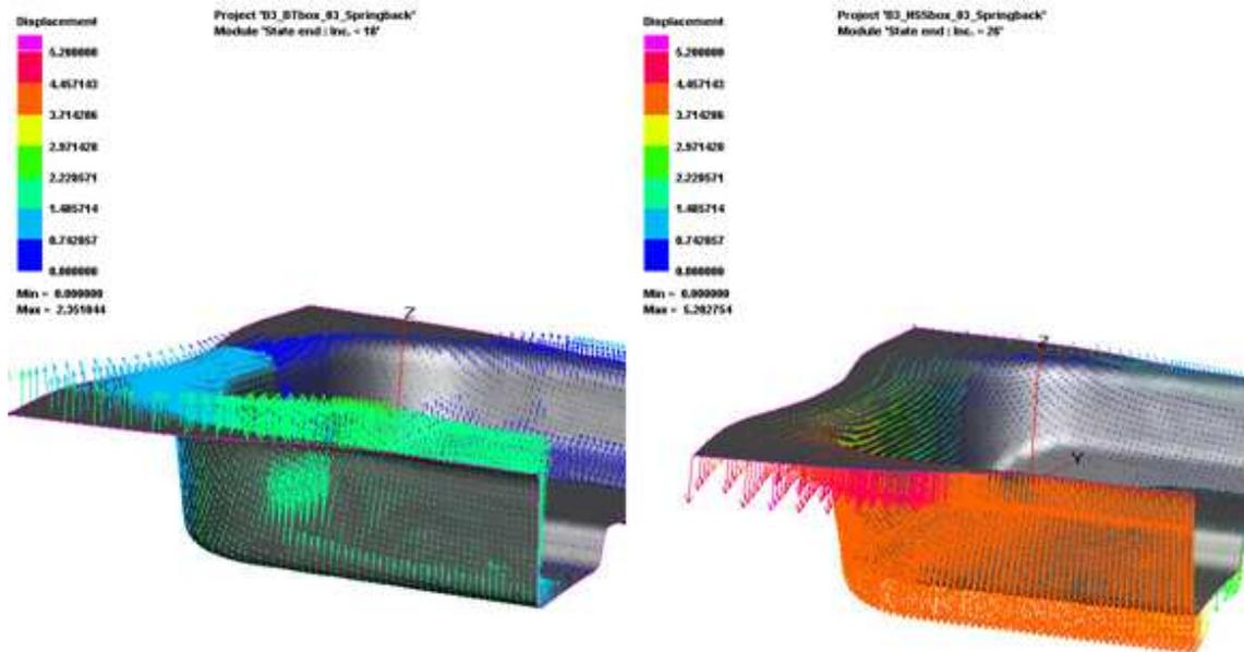
Figure 10: result of the calculation of the test case. Left side, the traditional shell element, right side the new normals stress shell.
