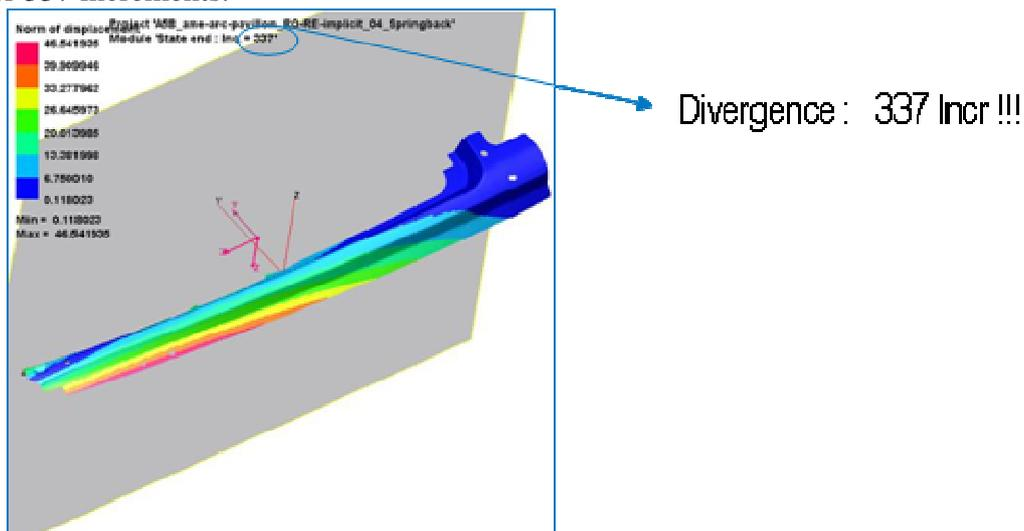
*Figure 1: Sample where the traditional springback calculation fails.*
