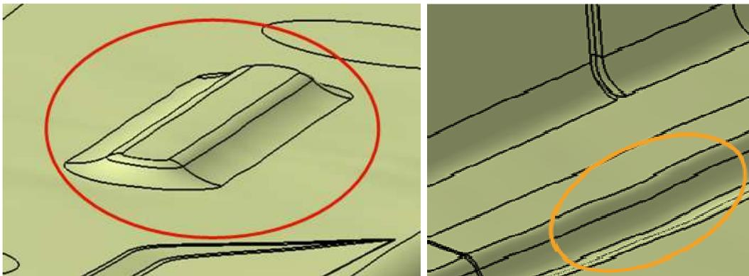
Figure 11: Samples of reconstructed surfaces where waves or bumps disturb the surface quality.
