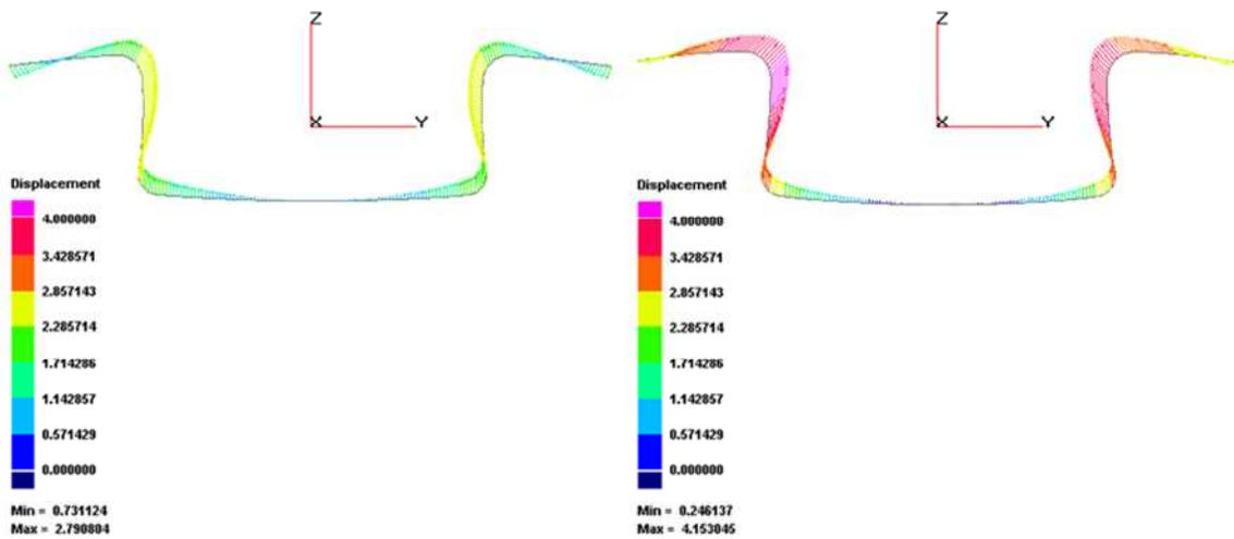
Figure 8: Test of the new normal stress shell element (left) compared to the normal shell element (right) – amount of springback
