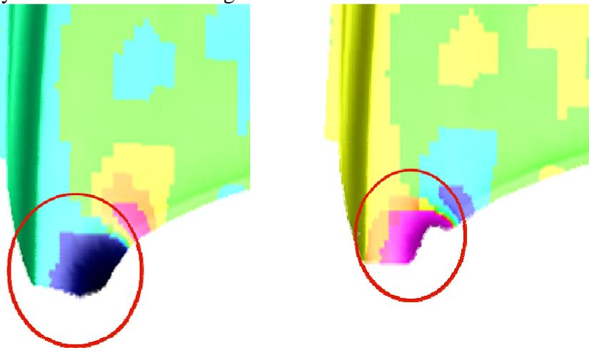
Figure 5: Using the new implemented methods for buckling analysis can in certain cases have a significant effect on the springback.
