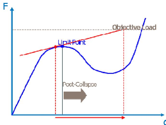
*Figure 3: Post collapse analysis after limit point.*
