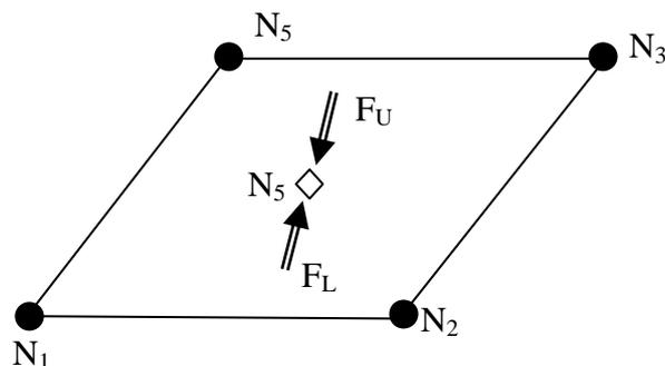
*Figure 7: New normal stress shell element with one additional virtual node.*
