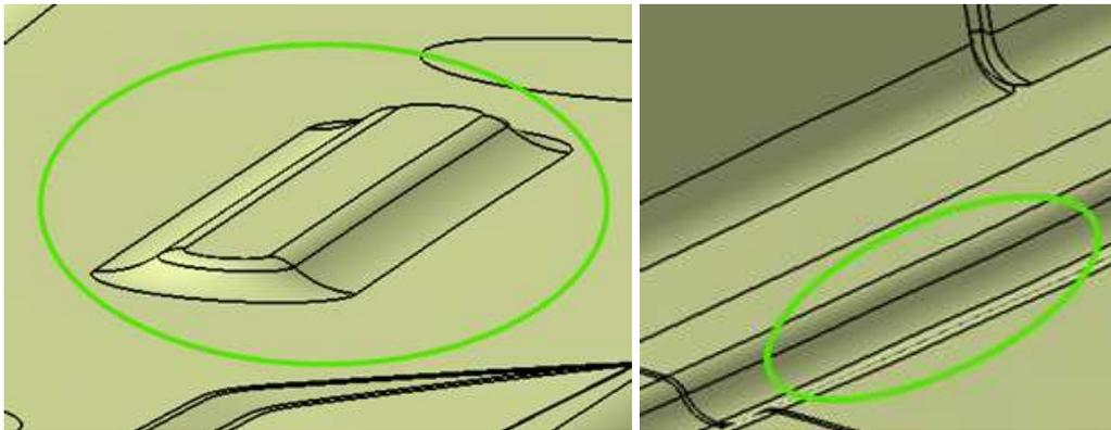
*Figure 12: Significantly improved surface quality after introduction of shape control during the springback compensation.*
