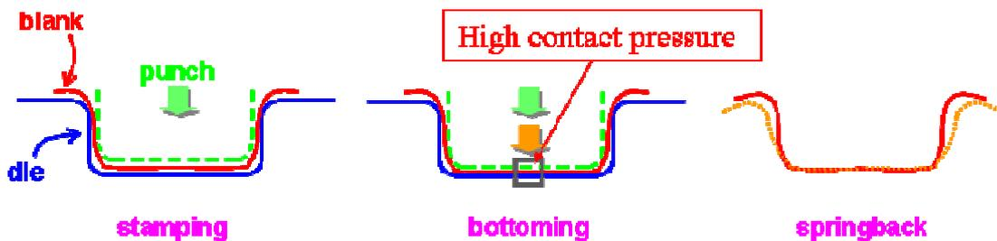
*Figure 6: If the stamping process is followed by a bottoming effect, this can have a (significant) influence on the springback*
