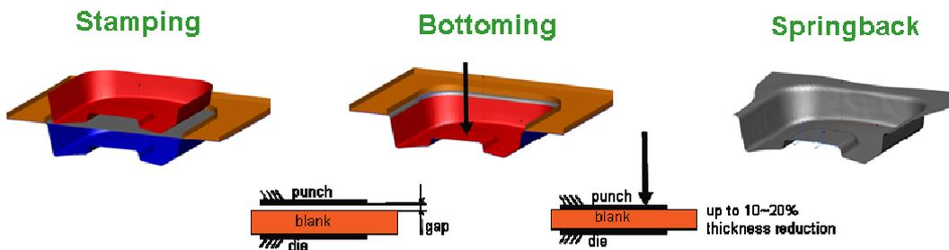
Figure 9: sample case for calculation of the bottoming effect on the springback.
