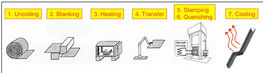
**Figure 2:** Schematic representation of hot stamping process.
