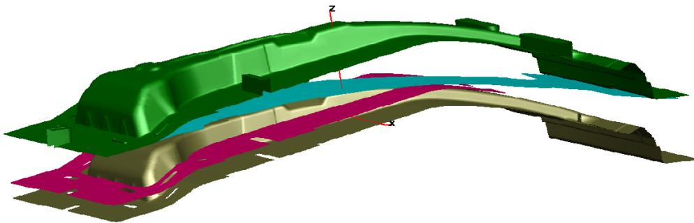
**Figure 6: Sample B-Pillar with tools, courtesy of AP&T**
