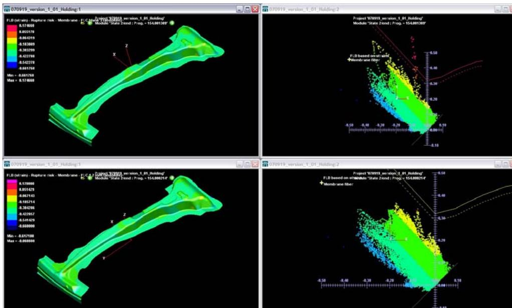
Figure 8: Comparison hot forming (bottom) to cold forming (top) – forming limit diagram
