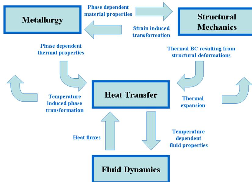
Figure 5: Different interactions during the hotforming process
