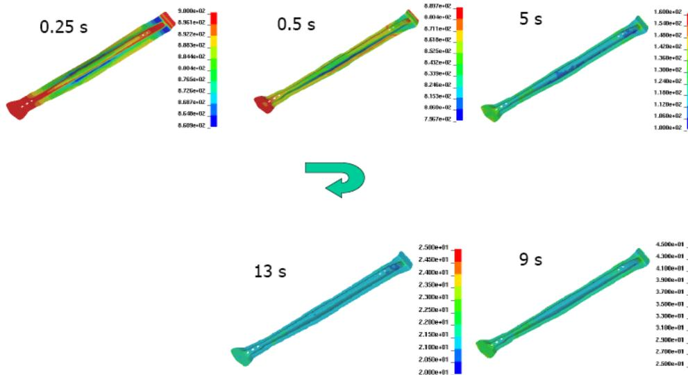
Figure 13: Quenching simulation [1] – temperature in the blank after the given number of seconds in the cooled tools.
