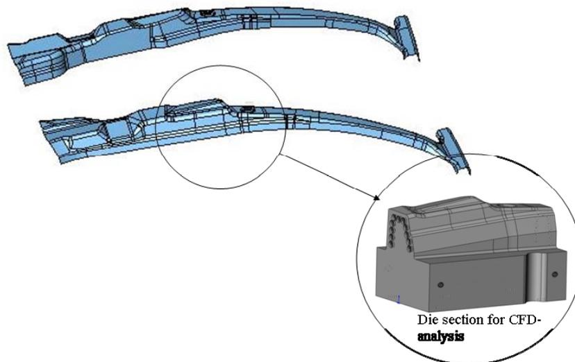
Figure 10: Section of the B-Pillar for CFD-analysis, courtesy of AP&T.
