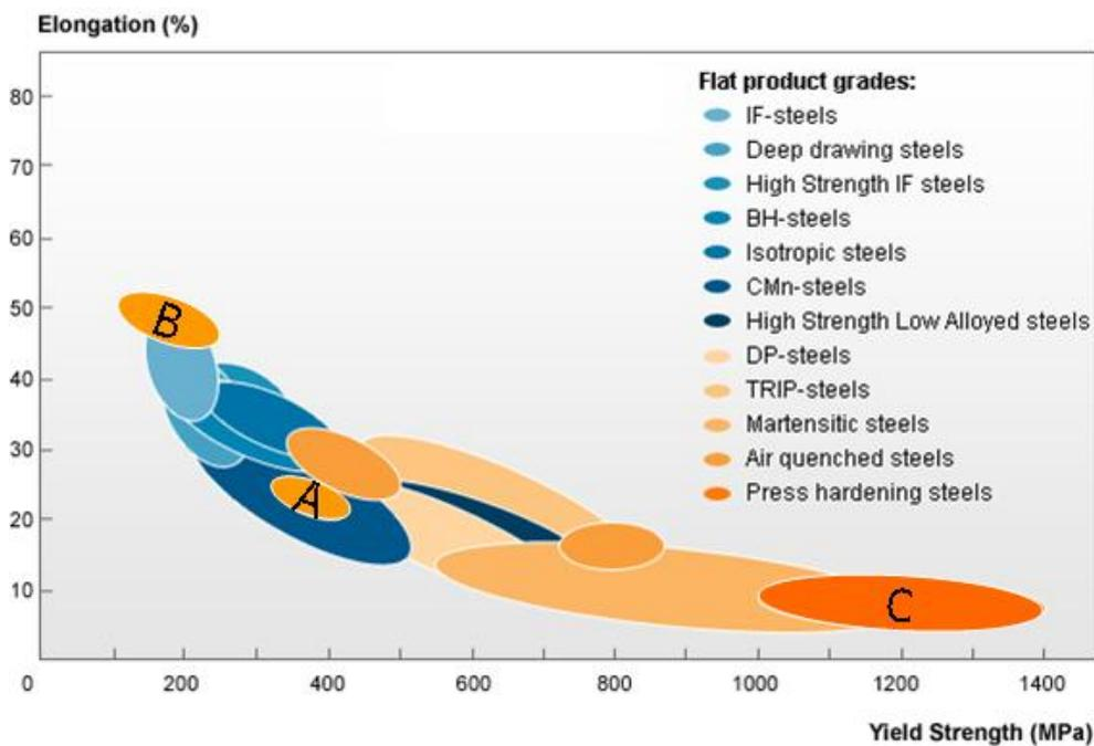
Figure 1: Typical hotforming material (Boron steel) A: as delivered; B: heated state – forming; C: after cooling: press hardened [1].
