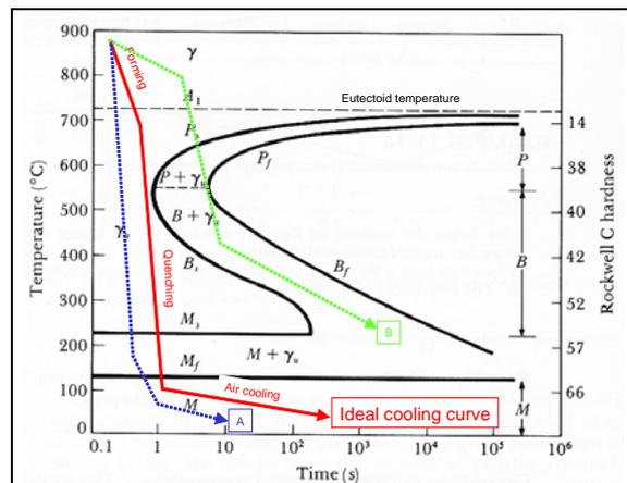
**Figure 3: TTT Diagram for a Eutectoid Steel together with possible cooling curves during hot stamping**
