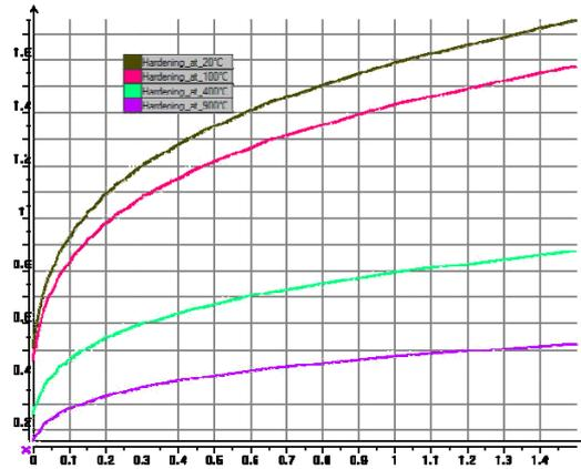
Figure 7: Temperature depending hardening curves
