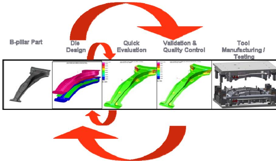
Figure 9: Working flow from part through die design, quick evaluation, validation to tool manufacturing [1].
