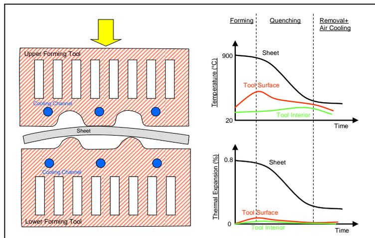
**Figure 4: Typical temperature evolution and thermal expansion during the hotforming process**
