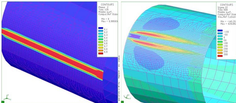
**Figure 15: Results of phase change simulation; left: martensite after cooling; right: residual stresses**
