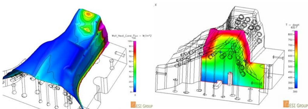
**Figure 12: Heat flux on the blank (left) and temperature distribution in the tool (right)**
