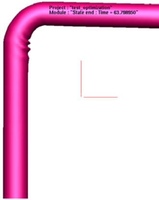
**Figure 10:** Strong wrinkling trend on the inner side with manual try-parameters.
