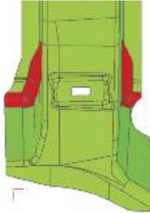
structural reinforcement for an automobile seat, explains that the part is made of high-strength steel and has a complex geometry that requires deep drawing. Further, the part becomes part of a spot-welded assembly and the weld area must be nearly flat.
