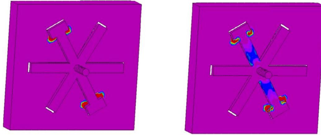
Figure 1: Accumulated Plastic Strain, Elastic Model (left) and Viscoplastic (right)
