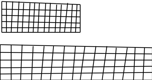
Figure 1: Enmeshment used in the modeling of a quarter of an ingot; top : 1100x500mm, bottom: 2200x600mm
