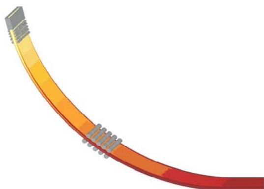
Fig. 10: thermal field during CC of steel (3D calculation, half of the strand)
