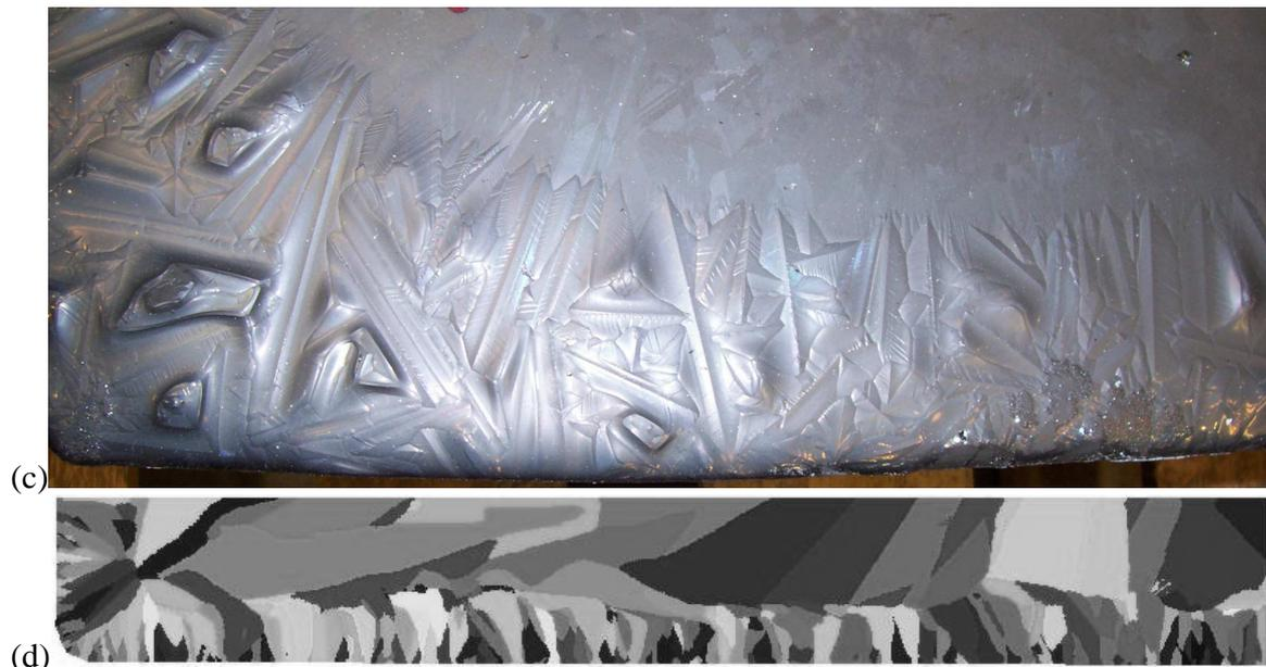
Figure 7. (a) Grain structure of the left half of the slab, (b) simulated grain structure of the right half, (c) grain structure of the top of a DSS ingot, (d) simulated grain structure of ingot top.
