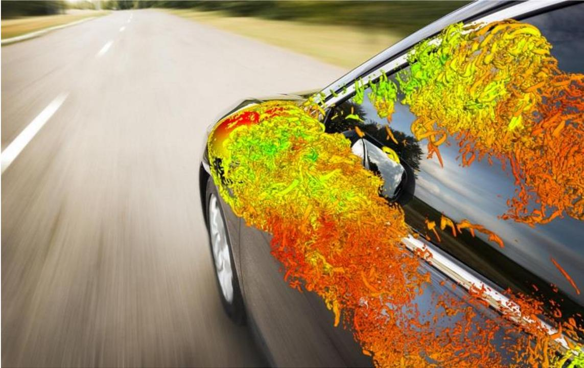
Image: Fluctuating surface pressures on the side glass of the car calculated using [OpenFOAM®](#) open source [CFD code](#). Complex, fluctuating surface pressure data can be imported into VA One from nearly any commercial CFD code.
