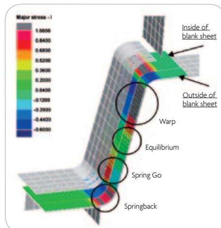
Stress components which cause springback
