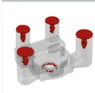
Fig. 1: The defects as seen in the initial castings before the change was made
