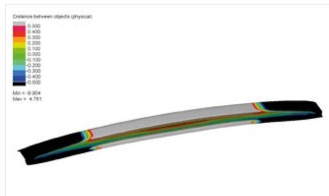
Fig.2 Initial distance between part geometry and springback.
