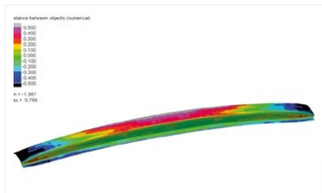
Fig.3 Final distance between part geometry and springback, after tool compensation.
