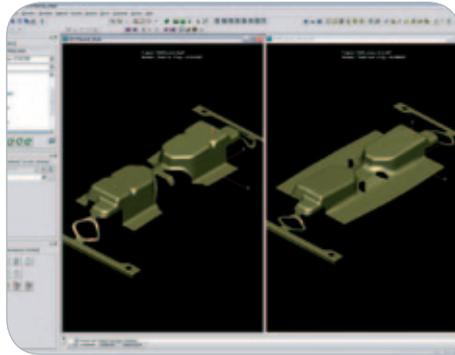
Cross-section of virtual die during forming simulation
