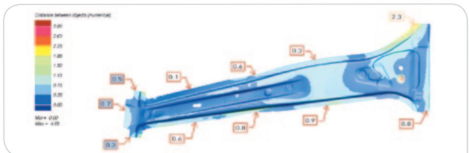
Figure 3: B-Pillar inner: PAM-STAMP 2G results with the Yoshida-Uemori model compare to physical testing.
