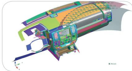
Fig. 3. The automated analysis also calculates target points and approach angles for head impacts.
