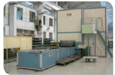
Real process environment of rubber pad forming
